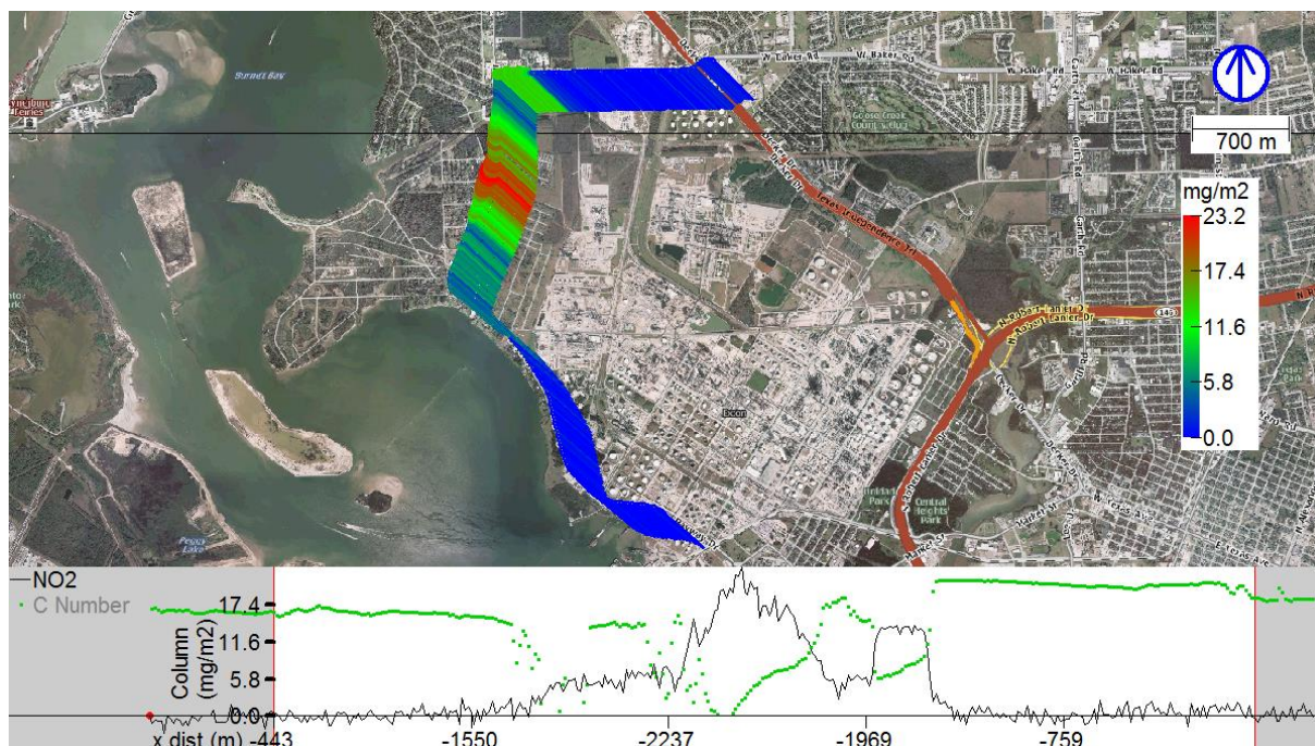
Figure 42 Mobile DOAS measurement of NO 2 northwest of Baytown (HSC 7) affected by clouds on September 8, 2013, 16:55–17:00. Each measured spectrum is represented with a point, which color and size indicate the evaluated integrated vertical NO 2 column. The NO 2 column by distance driven through the plume is also shown in the lower part of the figure together with the cloud indicator (green). A line from each point indicates the direction from which the wind is blowing.
