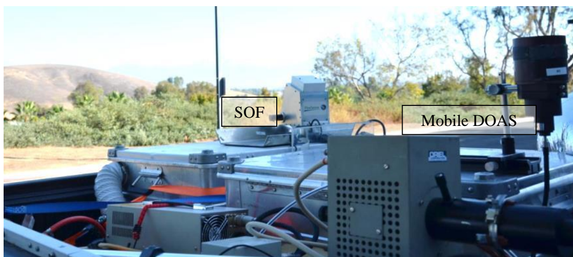
Figure 2 The SOF system. The solar tracker (front left) transmits the solar light into the infrared spectrometer (mid right with a GPS on top) independent of the vehicle's position.
