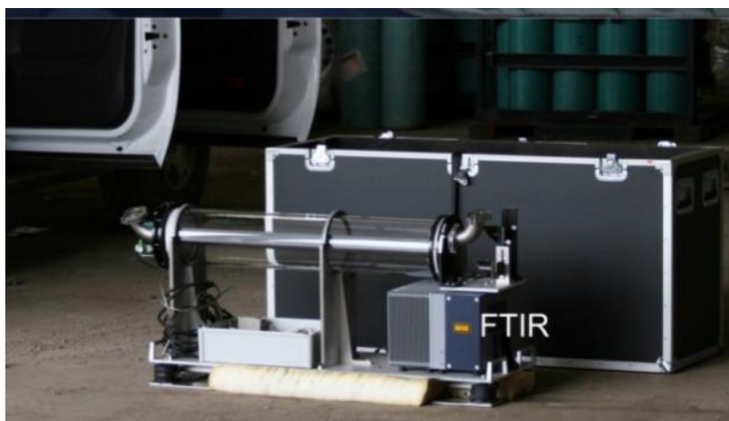
Figure 12 The MeFTIR instrument used in parallel with the SOF system during the campaign. The gas is extracted into the White-cell where it is analyzed by infrared absorption measurements. The residence time in the gas cell, and hence the measurements time resolution, is a few seconds.
